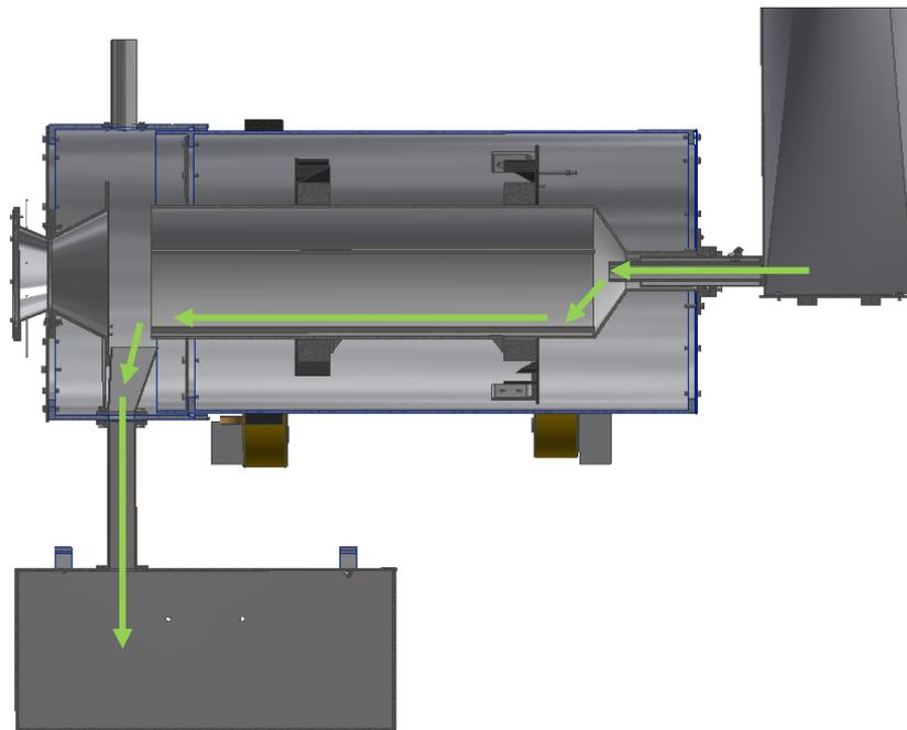
Figure 1: Schematics of the rotary kiln system and the storage.
